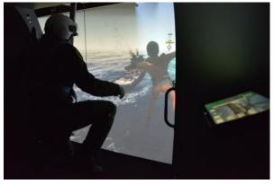
Mixed (simulated/ virtual) hoist on the right side Projection on a part of dome, centered on the eye of the crew member.
